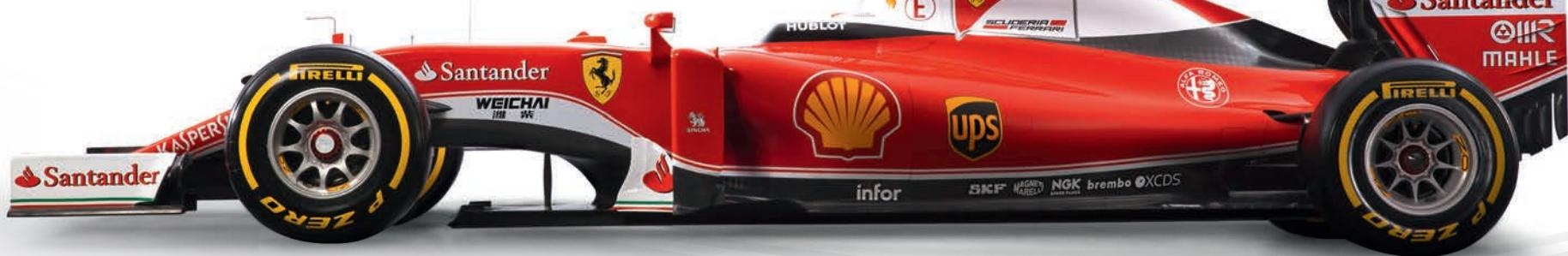
The SF16-H is the sixty second car built by Ferrari to take part in the Formula 1 World Championship. It is the third, since 2014 when the new rules were introduced, to be powered by a hybrid power unit, featuring a turbocharged engine fitted with two electric motors, one fitted directly to the transmission and the other mounted on the turbo shaft.
